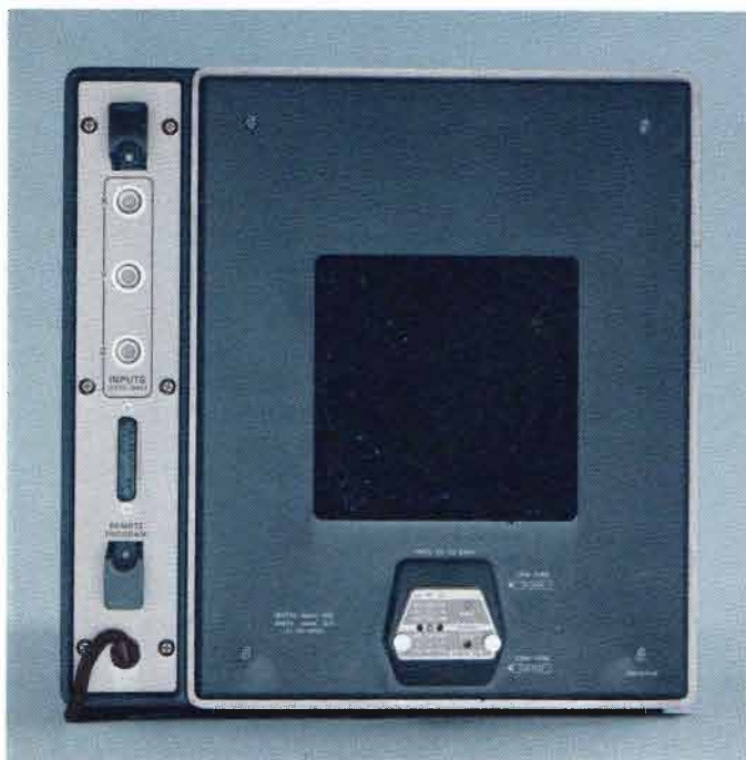
Rear panel of Type 611 Storage Display Unit.
