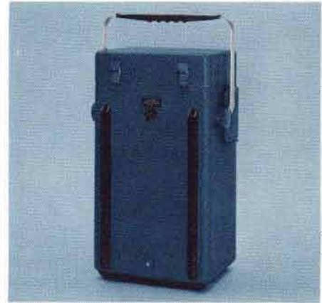
Type 453 MOD 165M with watertight front-panel cover in place.
